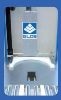
The possibility of choosing dies of different diameters allows optimal centering of the paint bucket.
